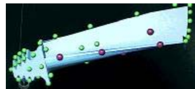
The easiest check was to generate spheres the same diameter as the probe ball at each of the digitized locations. Green spheres touch the CAD drawing as expected, but red spheres are oversized, which indicates
