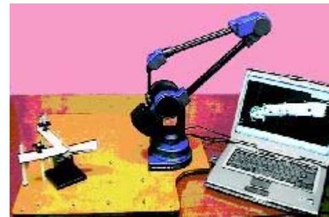
The MicroScribe MX system accuracy is said to be 0.004 in., but many of the digitized points can be within 0.003, 0.0002, or even 0.001 in.
